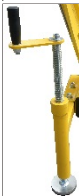
Stabilizing platform mechanism
